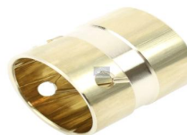
YSM 137 BPW CAMSHAFT BUSH ROR MERITOR (43x48x50) OEM NO. 21209990
