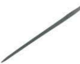
YSM.A 382 BALE SPEAR 39"-NORMAL Dimensions Length - 982.7 mm Thickness - 44.8 mm Threads - M30 X 2.0 RH Surface Finish - Grey Paint Heat Treated
