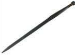
YSM.A 376 BALE SPEAR 27" Length - 685.8 mm Thickness - 36.36 mm Threads - M20 X 1.5 RH Surface Finish - Grey Paint Heat Treated
