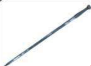
YSM.A 384 BALE SPEAR 49"-NORMAL Dimensions Length - 1238.25 mm Thickness - 44.8 mm Threads - M30 X 2.0 RH Surface Finish - Grey Paint Heat Treated
