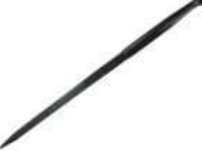
YSM.A 383 BALE SPEAR 39"-HEAVY DUTY Dimensions Length - 984.25 mm Thickness - 45 mm Threads - M30 X 2.0 RH Surface Finish - Black Paint Heat Treated
